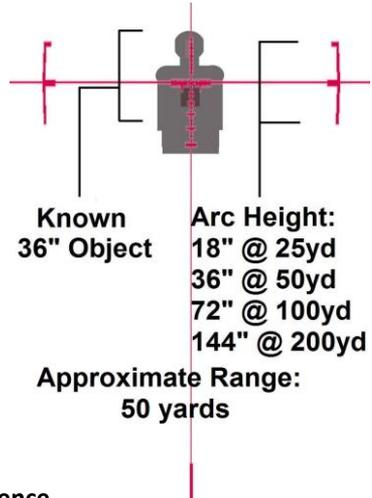
At 1x, use the large outer arcs as a fast reference to acquire and center the target for engagement.
